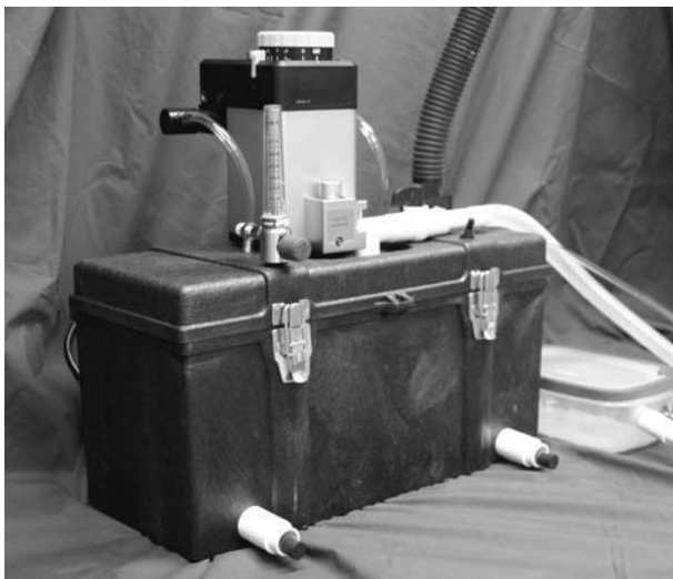
Fig. 5-38 Multistation Rodent Anesthesia Delivery and Scavenging System. This compact machine is shown with a vaporizer at the top of the case. Two coaxial delivery cones are at the bottom corners. An induction chamber is seen at the right and the waste gas transfer hose at the top right, near the vaporizer. Credit: Courtesy of BioTex.
