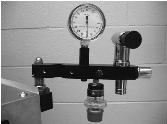
Fig. 5-19 Modified Mapleson-D Arm. In this photo, the Mapleson-D arm has been modified by the addition of a positive end expiratory pressure (PEEP) valve located below and between the APL valve and the circuit manometer. The PEEP valve provides an adjustable safety pressure release to the system. Credit: Courtesy of David S. Hodgson, D.V.M., DACVA.
