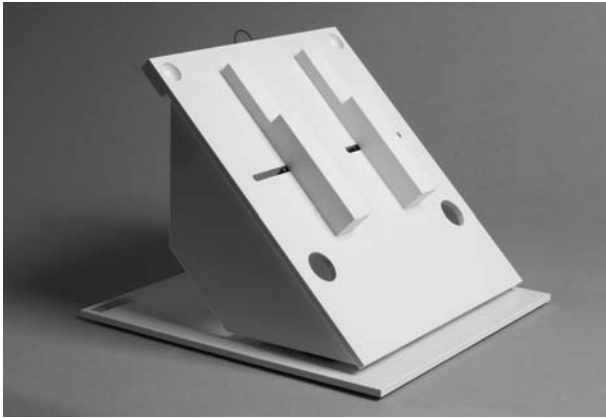
Fig. 5-42 Hallowell Rodent WorkStand. The stand is seen tilted to the 45° angle used during intubation. The adjustable lateral positioning aides are in the center, rotated to accommodate mice. The holes at the base and the depressions at the top are for a tube of 1/8 inch umbilical tape, used to secure the endotracheal tube in rats, and lidocaine gel used for mice, respectively. Credit: Courtesy of Hallowell EMC.
