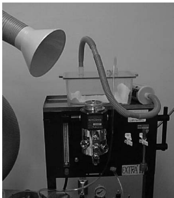
Fig. 7-1 Example of simple “snorkel apparatus” for active WAG evacuation placed at the induction-box opening.
