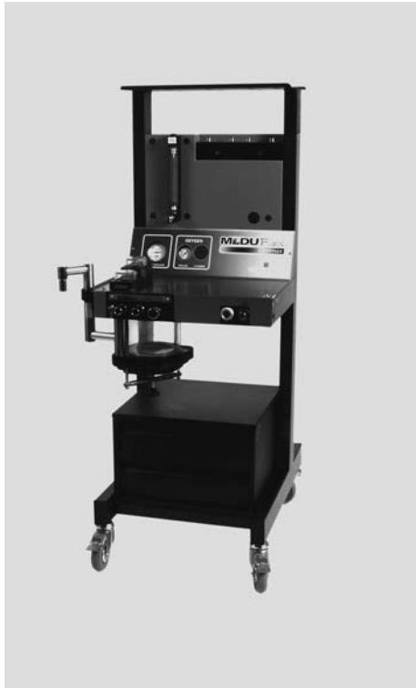
Fig. 5-25 Dipomed Optimax Elite. This model has a large workspace, a monitor shelf, and mounts for three flowmeters. Lockout mounts for two vaporizers are located to the right of the flowmeters. To the left, on the angled panel below the flowmeter assembly, is a breathing system manometer adjacent to two pipeline pressure gauges. The unidirectional valves are mounted on the workspace in front of the breathing system manometer. Breathing circuit connections and the oxygen flush valve are mounted on the face of the workspace and the absorber assembly is mounted below, as are two drawers in the base. Credit: Courtesy of Dipomed Ltd.
