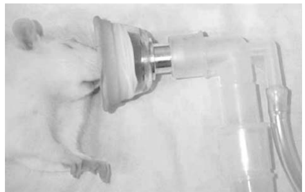
Fig. 7-3 Example of simple engineering controls that could be utilized to mitigate occupational exposure to WAG in the research setting: a homemade diaphragm is manufactured from the thumb portion of a small latex surgical glove. The thumb is removed using scissors and then stretched over the orifice of a conventional conical rodent face mask, creating a small (0.5- to 0.8-cm long) aperture just large enough to contain the animal's nose.
